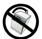
Do not overturn the machine after installation (e.g. for maintenance purposes). This could lead to a malfunction of the device controlling the water level in the wash chamber. Should the machine be overturned accidentally, follow the instructions given in the section "SERVICING AND REPAIR" to restore correct operation.
